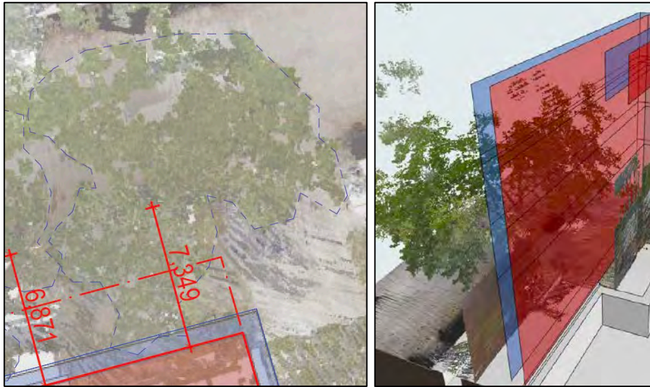
Figures 61 & 62: The Tree canopy impact of the proposed building in Pink and 1m wide scaffold in Blue. (Source: Tree Canopy Modelling by Plus Architects dated 1/08/2023)
